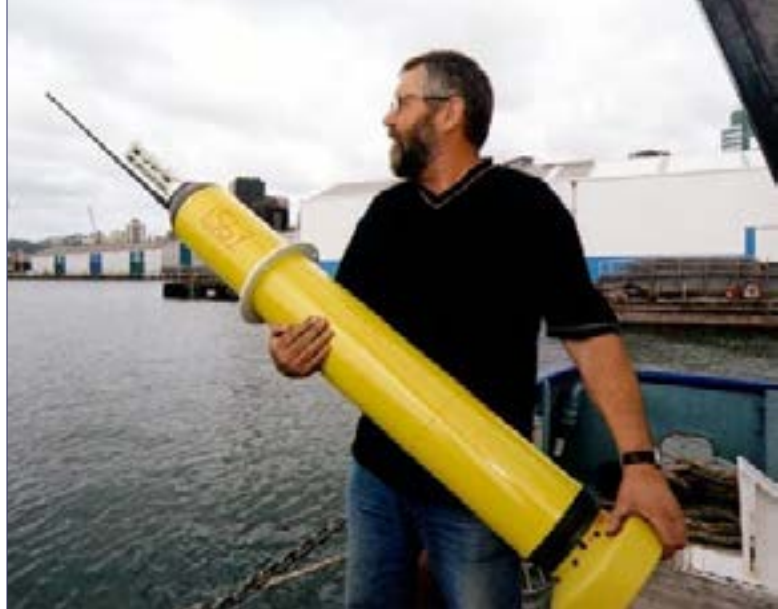
An Argo smart float is readied for the ocean. When the Argo global network is complete, it will include 3,000 free-drifting floats that can measure the salinity and temperature of the ocean's top two kilometres. New Zealand research vessels released more than 100 Argo floats into the sea in 2003–4; NIWA.
