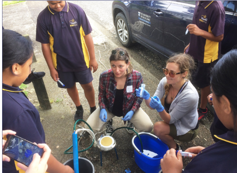
University of Auckland PhD students Emilie Glos (left) and Olivia Mosley set up a pump attached to a car battery to filter local stream water through a 0.2 µm mesh to collect organisms, talking with Tamaki Primary School students who took the water samples.
