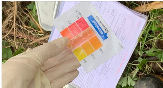
Checking nitrate levels in the sample tube.
