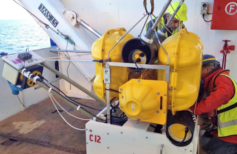
A device including an ocean bottom seismometer and an absolute pressure gauge is checked before being dropped to the sea floor, as part of the HOBITSS experiment. Photo: Erin Todd.
