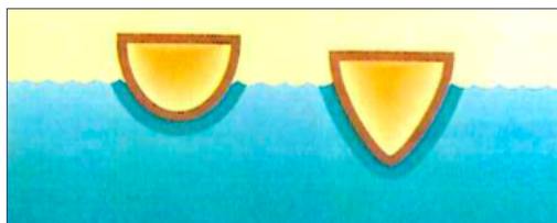
A U-shaped hull for a coastal, paddled waka, and a V-shaped hull for a waka hourua sailing the Pacific from Hawaiki. From Applications booklet .
