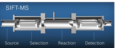
A simplified the SIFT-MS instrument; the flow tube is where the reaction happens.
