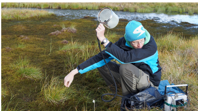
Christian measuring plant photosynthesis and carbon dioxide (CO 2 ) exchange, using a portable CO 2 chamber system.
