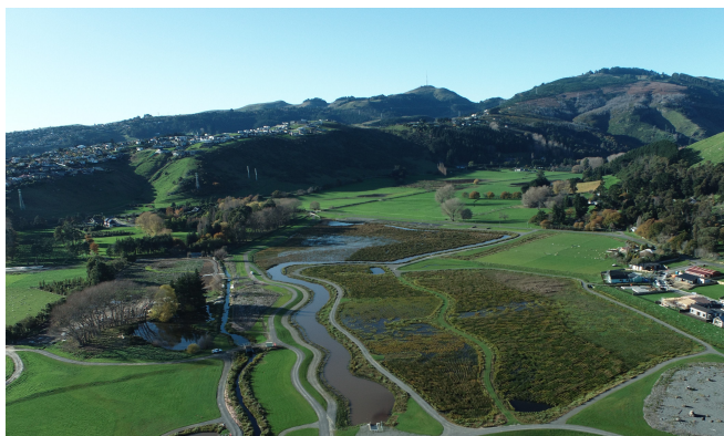
Pictured above is Te Kuru wetland, a project that Stephanie worked on. It is a 109-hectare stormwater facility featuring expansive wetland areas, stormwater storage, and filtration basins. Courtesy: Stephanie Dijkstra
