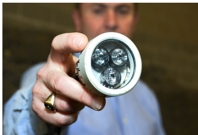
ABOVE: LED for miners, to increase visibility inside mines [National Institute for Occupational Safety and Health]
